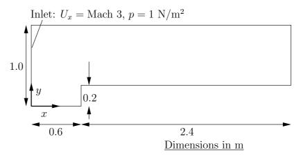
Figure 3.7: Geometry of the forward step geometry
