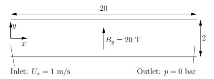
Figure 3.12: Geometry of the Hartmann problem
