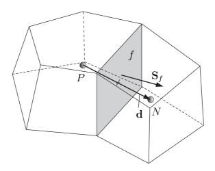
Figure 2.2: Parameters in finite volume discretisation
