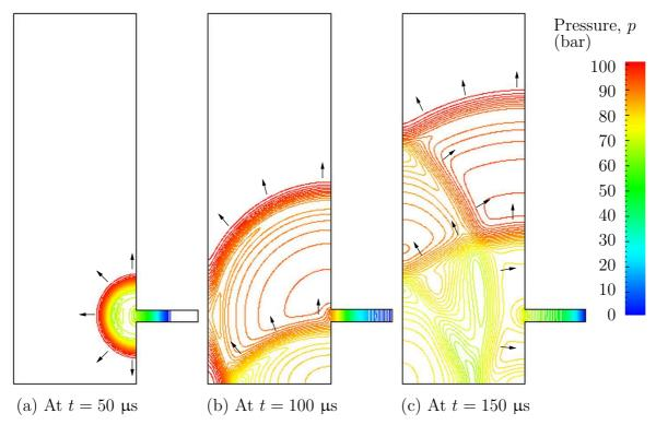
Figure 3.11: Propagation of pressure waves with refined mesh
