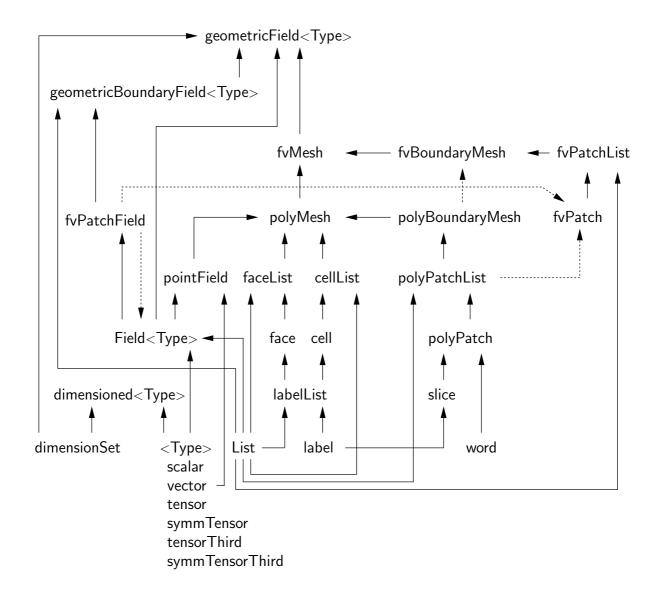
Figure 2.5: Basic class structure leading to geometricField<Type>
