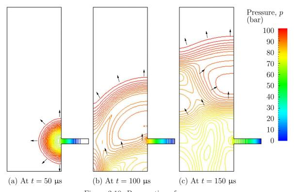
Figure 3.10: Propagation of pressure waves
