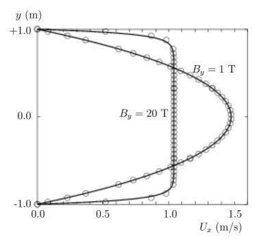
Figure 3.13: Velocity profile in the Hartmann problem for  $B_y=1~\mathrm{T}$  and  $B_y=20~\mathrm{T}$ .
