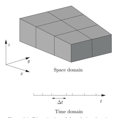
Figure 2.1: Discretisation of the solution domain
