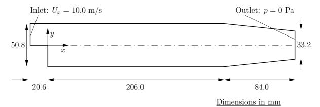
Figure 3.4: Geometry of backward-facing step
