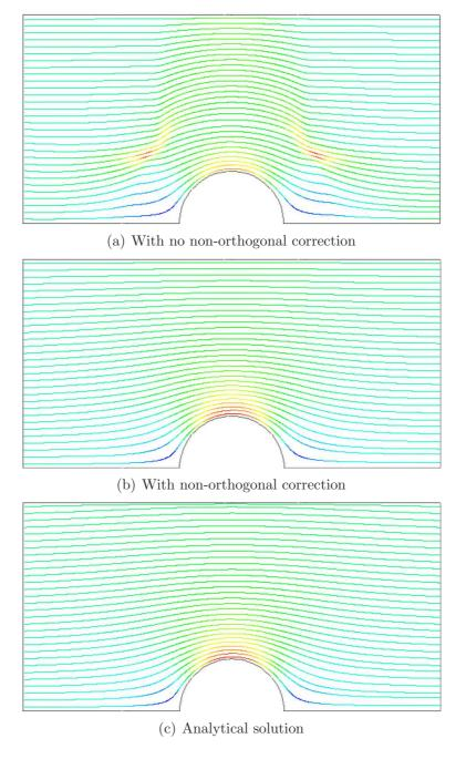
Figure 3.3: Streamlines of potential flow
