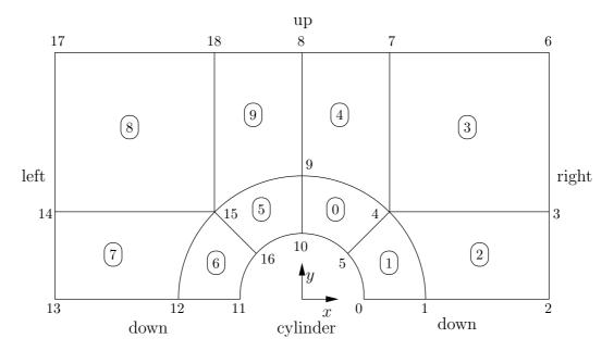
Figure 3.2: Blocks in cylinder geometry
