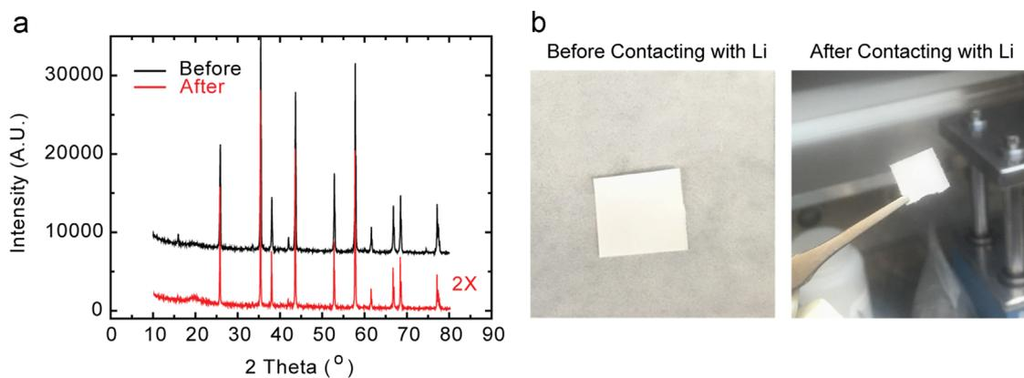
**Figure 6** Stability of Al<sub>2</sub>O<sub>3</sub>/polymer separator against lithium metal. The composite separator is attached to lithium and soaked in 1 M LiPF<sub>6</sub> in EC/DEC for seven days. (a) XRD pattern before and after contacting with Li. (b) Optical image of a composite separator before and after contacting with Li. No change has been observed. It is supposed that polymer coating effectively block direct reaction between lithium and Al<sub>2</sub>O<sub>3</sub>.
