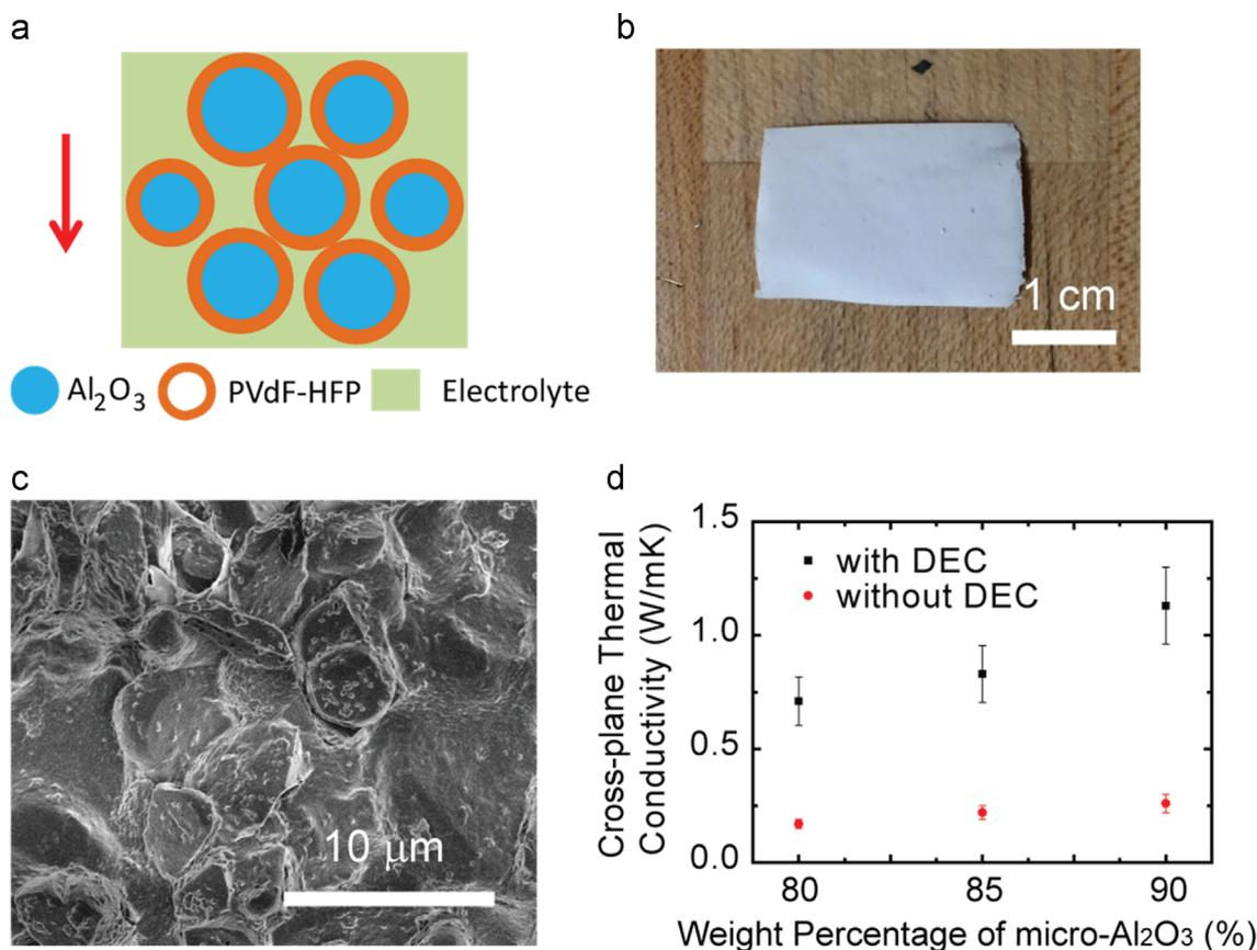
**Figure 3** Micro- $\text{Al}_2\text{O}_3$ /PVdF-HFP composite separator. a) A schematic of micro- $\text{Al}_2\text{O}_3$ /PVdF-HFP composite to improve thermal conductivity of a separator. b) and c) Optical and SEM images of the composite separators. The particle size is  $\sim 10 \mu\text{m}$ . The weight ratio of micro- $\text{Al}_2\text{O}_3$  to PVdF-HFP is 85:15. d) Cross-plane thermal conductivity of the micro- $\text{Al}_2\text{O}_3$ /PVdF-HFP separator.
