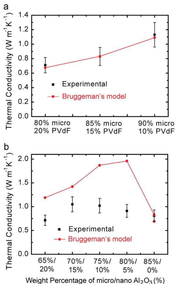
**Figure 5**  $k_{eff}$  of the composite separator calculated by the Bruggeman's model. a) Micro- $Al_2O_3$ /PVdF-HFP composite separators. b) Nano/micro- $Al_2O_3$ /PVdF-HFP composite separators. The weight percentage of PVdF-HFP is fixed as 15%.
