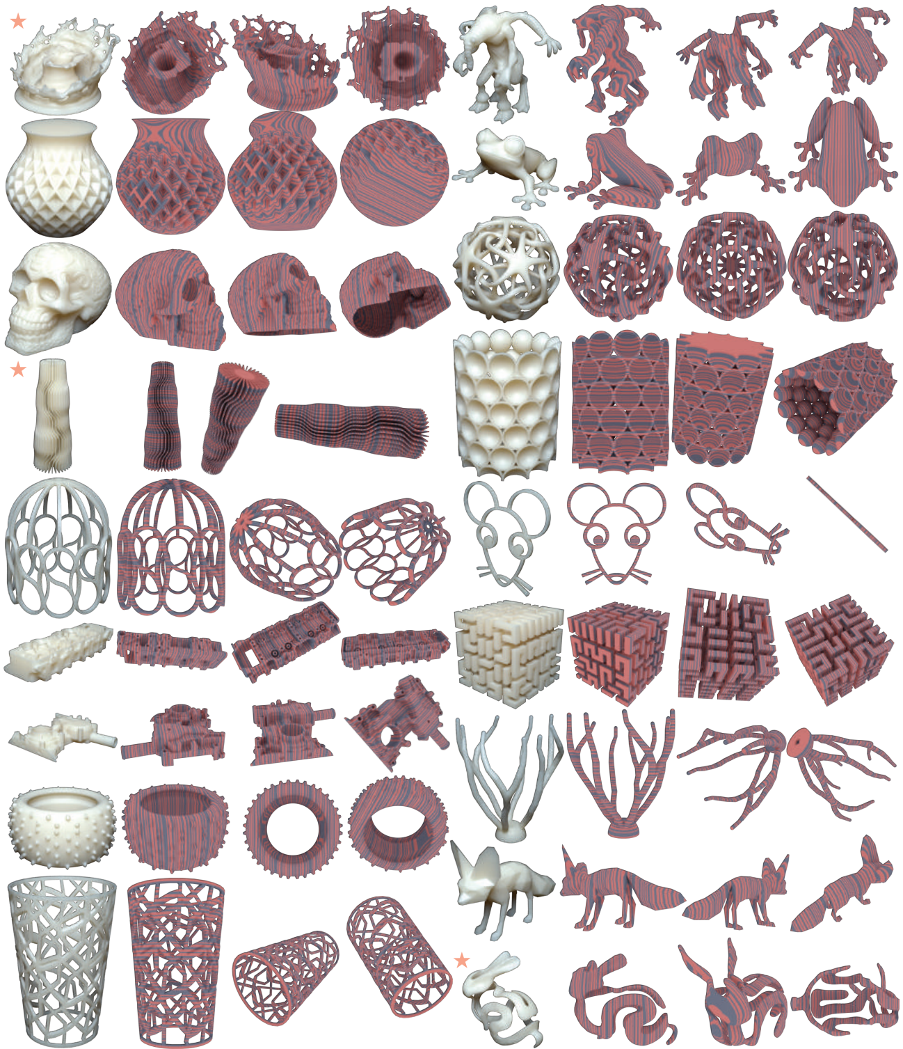
Fig. 23. Successfully decoded shapes. A peek into the diversity of tested shapes within our database. Each view presented is correctly decoded by our graph-based algorithm. Shapes with bumpy, shell, thin, curvy, and other challenging properties showcased here are still subject to encoding and decoding by our LayerCode approach. Three shapes indicated by the stars are discussed in the main text.
