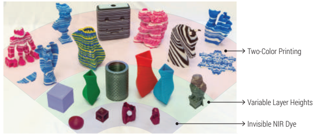
Fig. 11. Fabricated pieces carry LayerCode tags made by two-color printing, variable layer heights, and near-infrared resins. LayerCode tags are successfully tested on bumpy, shell, curvy, and otherwise complex geometry.
